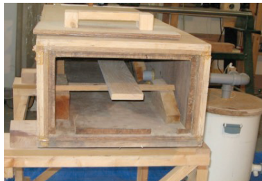
Photo 4-3. The workpiece is placed inside the steam chest and raised off the base ready for 6 hours steaming. The boiler shown holds 30 litres of water which generates a constant flow of steam without requiring replenishment during the 6 hours steaming period.
