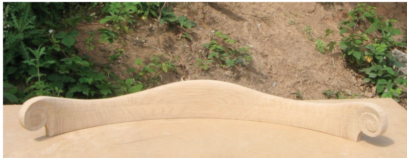
Photo 4-26. The completed oak crest piece made from three cut-out's of 30mm thick sawn oak board. The three pieces were glued up to form the workpiece (See photo 4-30) from which this crest was made.
