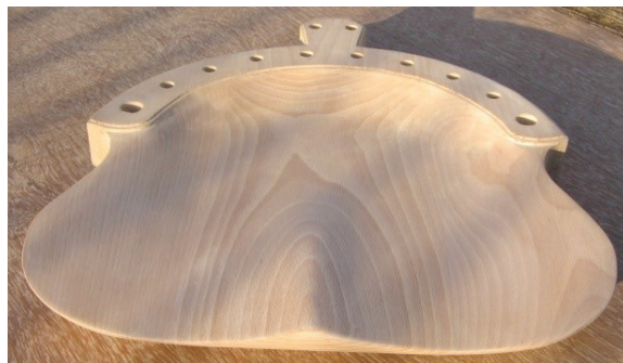
Photo 3-44. The Figure shows another seat made in European Beech, completed in accordance with the same procedures of these chapters, but with the hollow finished to the deeper levels of Figure 33, with a maximum depth of 26mm.
