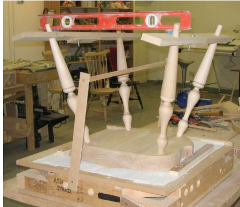
Photo 5-4. The set-up now includes the MDF leg ties with the spirit level, packed up on blue packers, to 16.5 inches (419mm) above the seat across the front legs.
