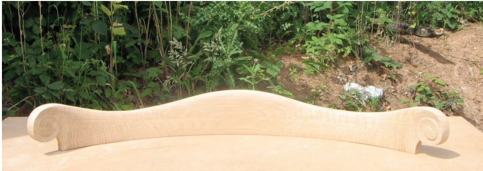
The crest piece made from three pieces of oak glued together. See chapter 18 of this part for making a crest piece without the need to steam and bend.
