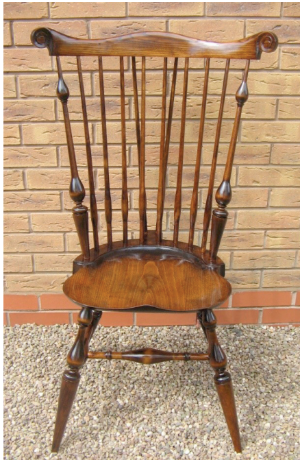
Photo 1-7. American Windsor side chair. The crest is American white ash, the seat European beech and the spindles are made from hard rock maple. The stain is oil based brown mahogany followed by one coat white shellac sealer and two coats of French polish. A third coat of French polish was applied to the seat and crest. The water based stain shown in photos 1-1 and 1-2, also mahogany brown, gives a reddish tinge to the finished chair. But the oil based stain in this photo provides a colour that can be described as a rich brown.
