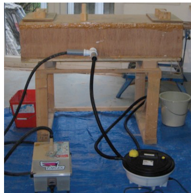
Photo 4-4. Two domestic steam cleaners are used in this set up for the generation of steam. Use one steamer at any one time which lasts for about 1 hour. The second steamer (shown for illustration purposes) takes over while the first steamer is replenished with water and made ready with steam.
