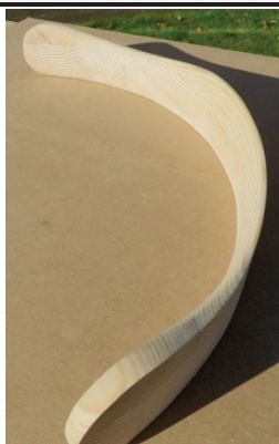
Photo 4-77p. Overhead view of the completed crest showing the slimline and splayed front face.
