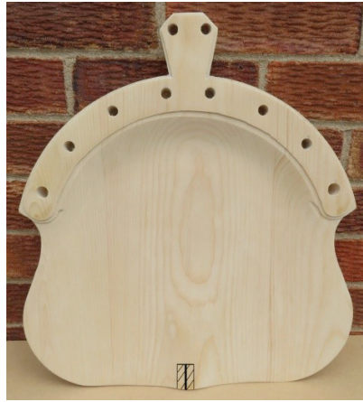
Photo 3-165p. The completed seat after final sanding. The 25mm flat top of the pommel at the front is retained for levelling the seat at the assembly stage.
