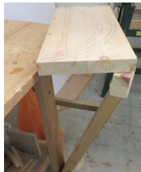
Photo 4-13p. Stage 2B. The Workpiece set up at the corner of the bench with the outside edge supported by a strut. Two screws secure the blank to the bench along the back edge. This arrangement allows all four cuts to be carried out without repositioning the workpiece.
