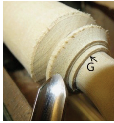
Photo 2-45p. Stage 3D. Shape the scotia. Shaping the scotia in progress.
